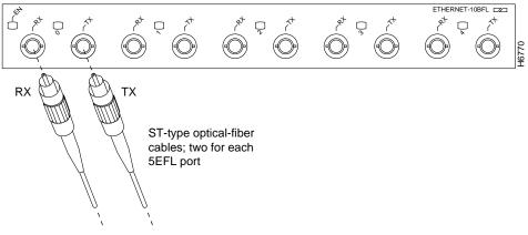
To the appropriate TX and RX ports of the repeater, hub, DTE or other external 10BASE-FL equipment
